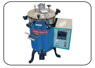
We offer is fully automatic Autoclaves are most useful to sterilize Lab Glassware, Plastic Tubing, Liquid in sealed glass containers, product contact & small critical equipment used in the aseptic formulation & parenteral drugs.
